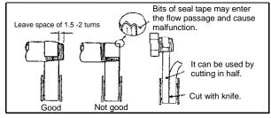
When installing piping or a joint, prevent penetration of chips or sealing agent. Also tightening torque should be within the range indicated below.
